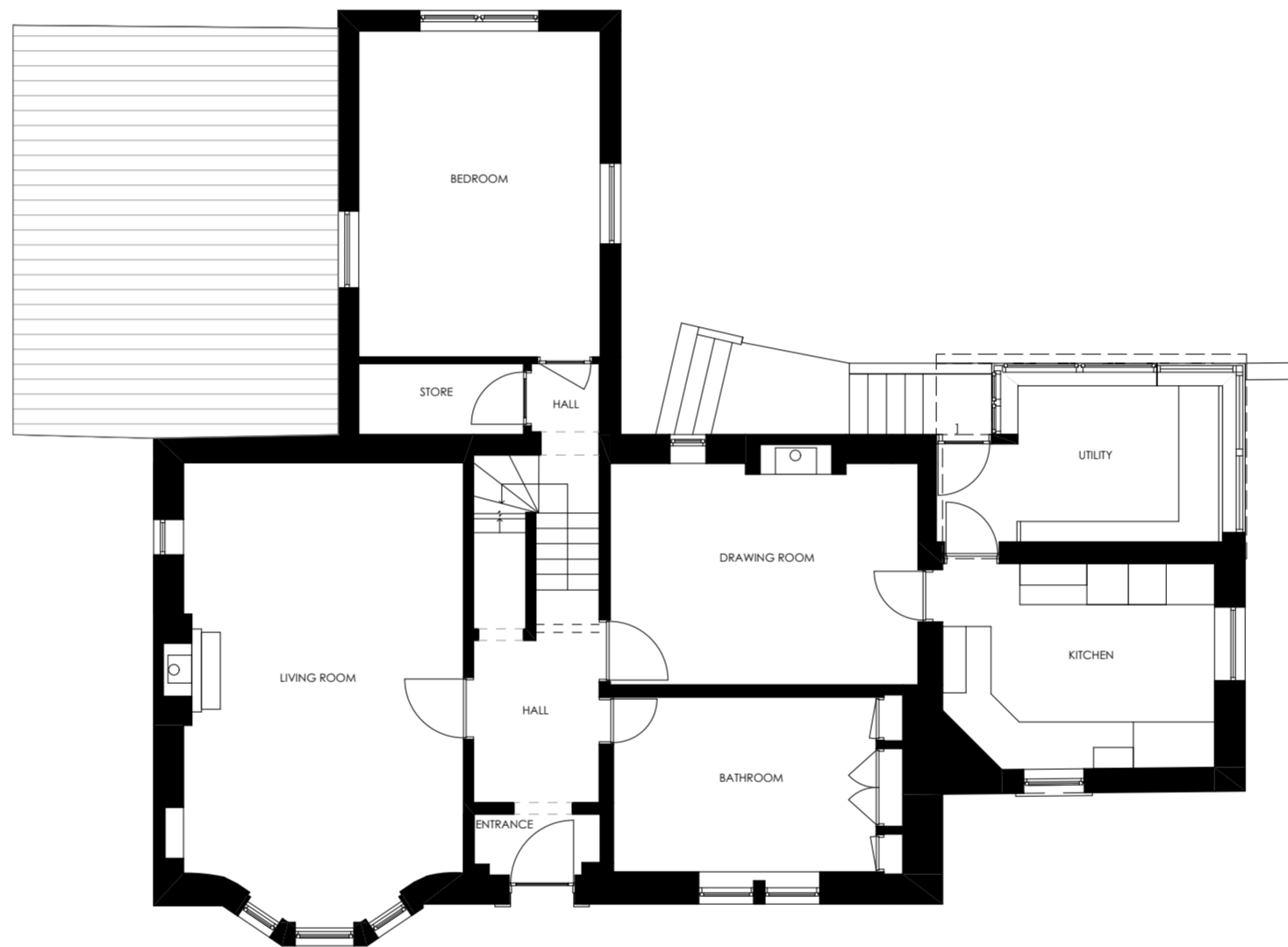
GROUND FLOOR AS EXISTING SCALES @ 1:100 (A2)
