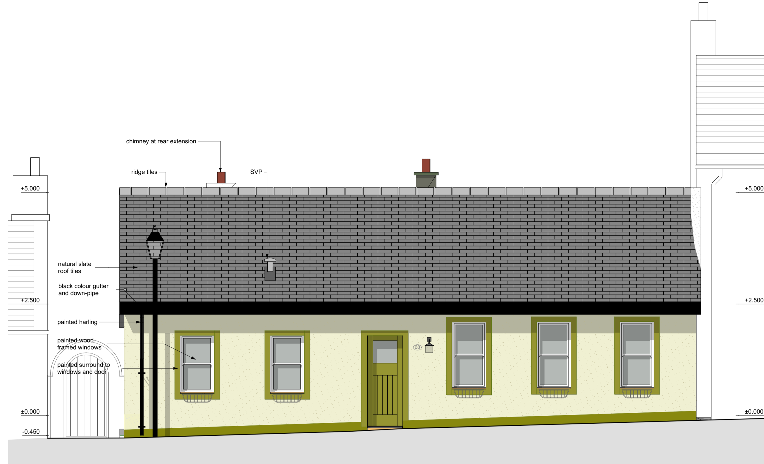
FRONT ELEVATION as Existing
