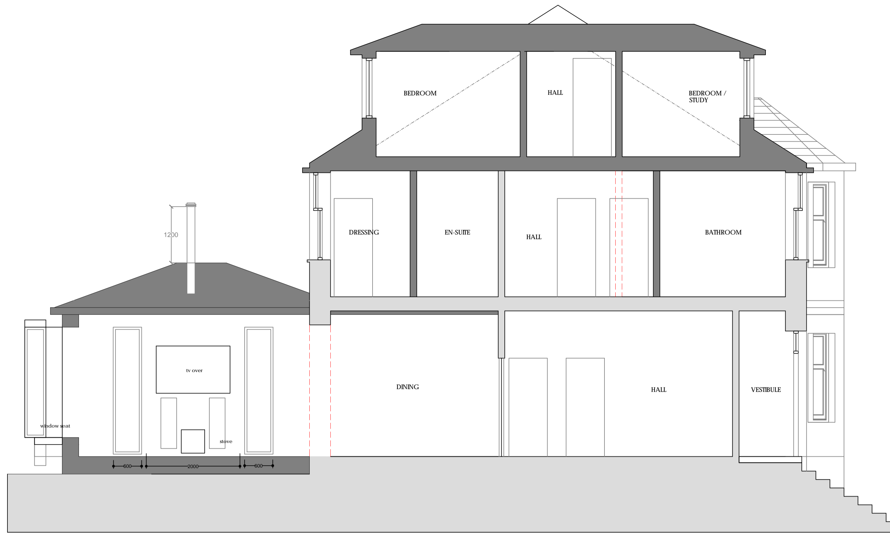
PROPOSED SECTION SCALE 1:100@A3 1:50@A1
