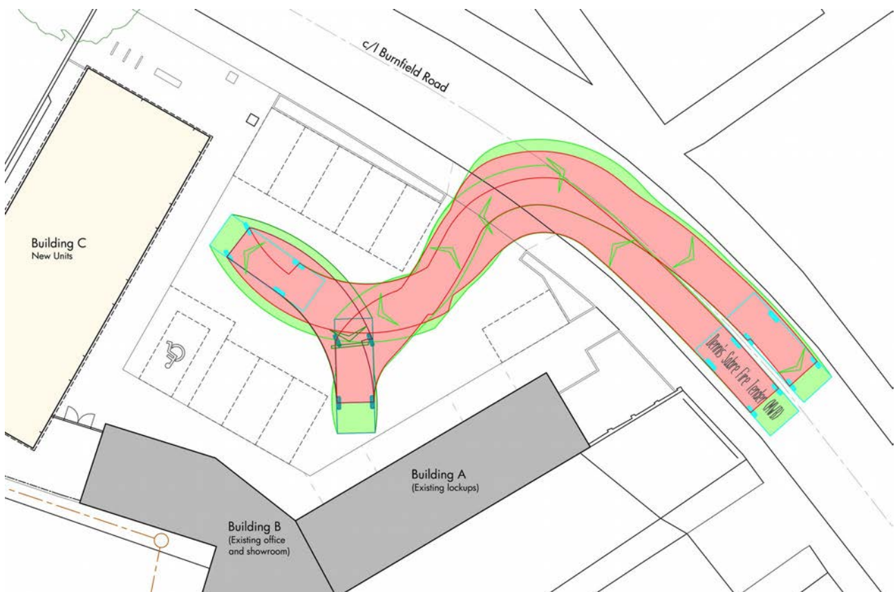
Swept path analysis showing fire engine entering and leaving site in forward gear.
