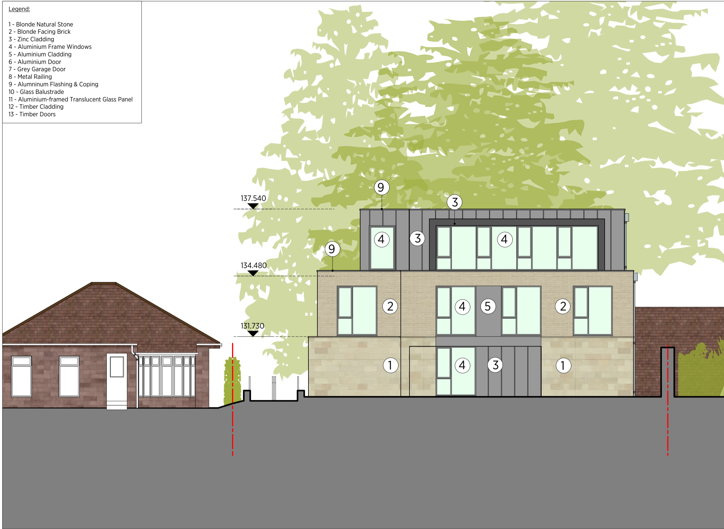
North - West Elevation as Proposed 1:100@A1/1:200@A3
