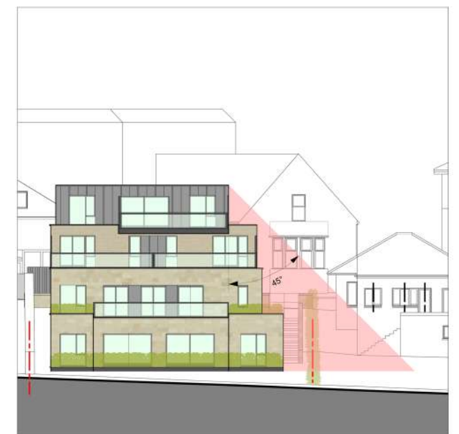
Sun Shading Elevation as proposed (45 degree approach). 1:200@A3 Possible Shading
