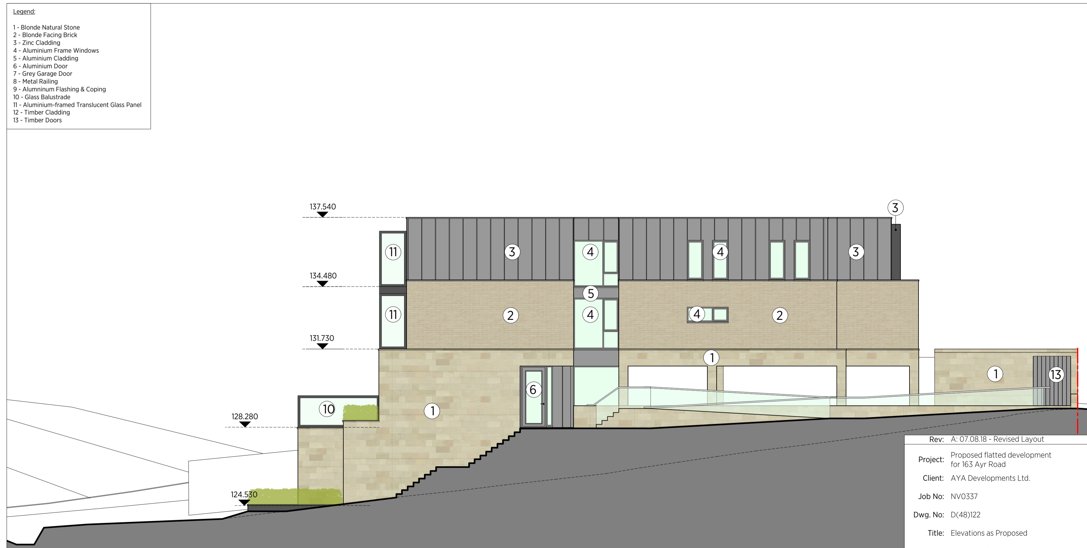
North - East Elevation as Proposed 1:100@A1/1:200@A3
