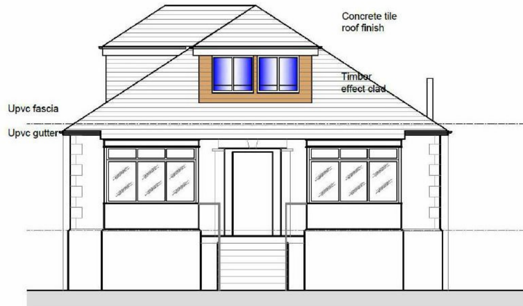
Front Elevation As Proposed
