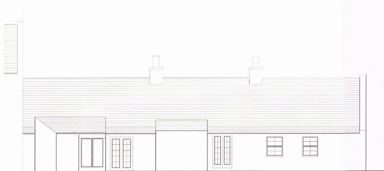
South East Elevation as Existing Scale 1:100
