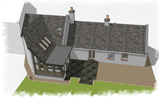
Illustration 10: The rear extension combines with the raised roof ridge to form a transition with the two-storey house next door, maintaining the style and character of the existing building but introducing a contemporary flavour
