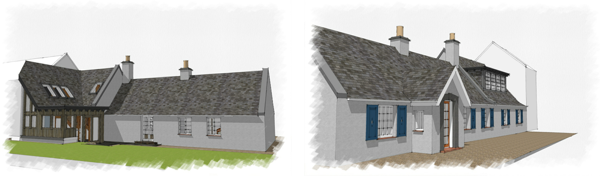
Illustration 13: Front and Rear views of the re-modelled West Crossgates. The combination of the raised roof ridge and the dormer reflect the history of the building by re-introducing the separation between the two original cottages as well as improving the transition and relationship between West Crossgates and the two storey building beside it. The alterations are appropriate to the character of the building and are an architecturally sound enhancement of the building and the streetscape. At the rear, the house creates a natural frame and enclosure to the garden while also creating a better architectural relationship with the adjoining two storey house.
