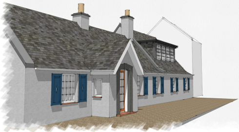
Illustration 3: The re-modelled front with the raised roof ridge stepping up towards No.44 together with the Georgian style dormer
