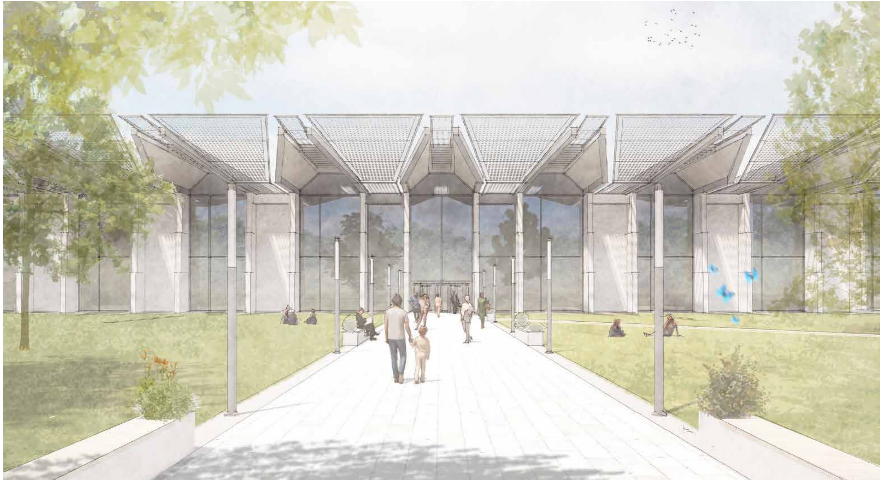
Preliminary Sketch Visualisation showing aspiration of glazing to woodland and roof canopies for solar shading and shelter
