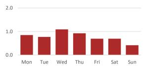
The amount of UFAS incidents have increased by 84% during this reporting period with a reduction of 8% over the 3 year average. The significant increase was caused predominantly by actuations at schools due to apparatus being contaminated by dust gathering within the detector heads due to the schools being closed and limited ventilation within.
