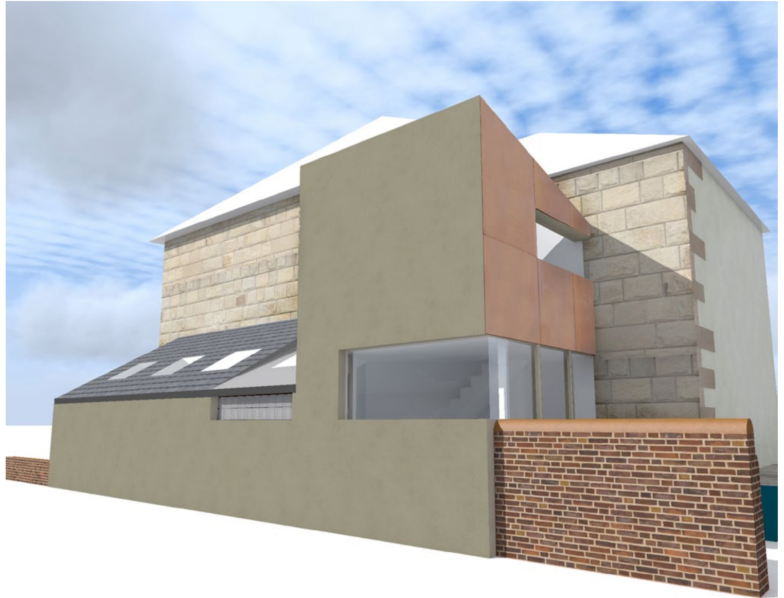
View from lane View showing render to side elevation and cor-ten steel to small gable facing garden
