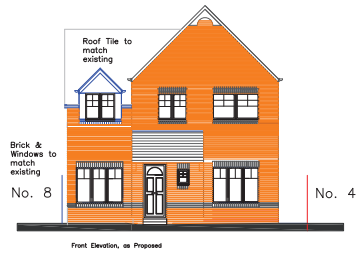
Front Elevation, as Proposed
