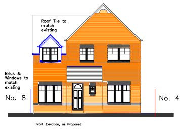
Front Elevation, as Proposed
