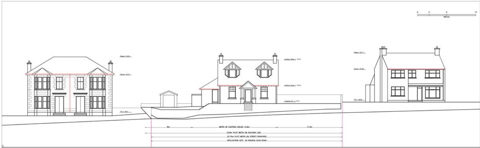
Contextual South-West (Front) Elevation as Existing @ 1:200
